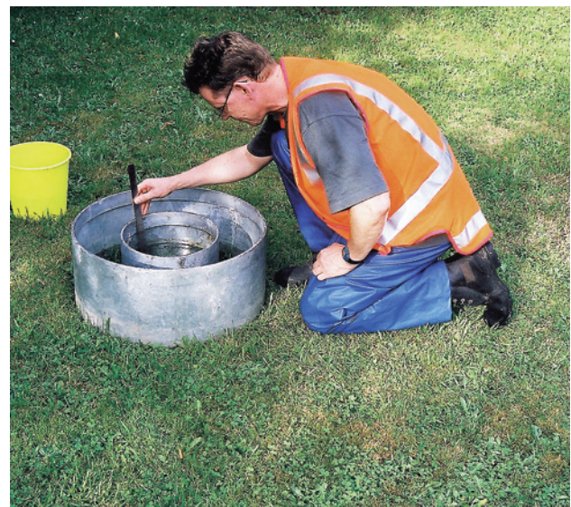
Figure 6-9: Double ring infiltrometer testing for measuring surface soil infiltration rates.
