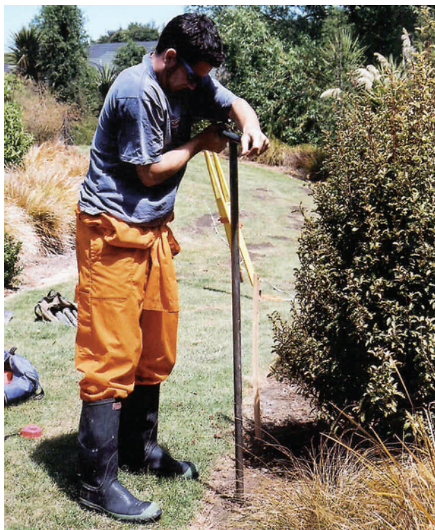
Figure 6-10: Inverse augerhole method for measuring surface and sub-surface soil infiltration rates.
