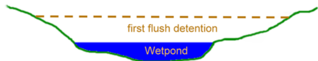
Figure 6-26: First flush detention area in relation to the wet pond area. For determining wet pond volume, the first flush detention requirement is additional to the required wet pond volume.
